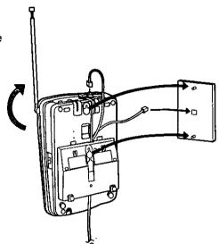
Pull down the handset hook until it locks, so the tab holds the handset.
