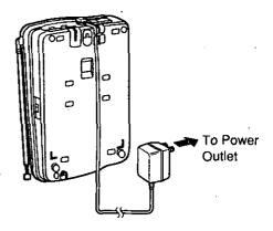
Tuck the telephone line cord inside the wall mounting adaptor.
